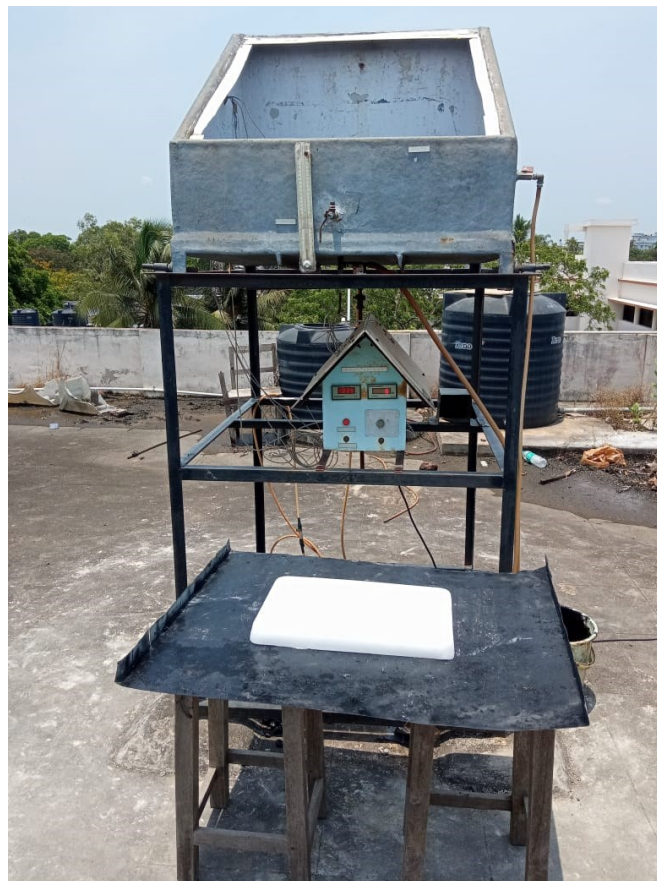
Fig 4.10 Photograph of solar still with wooden tetrahedrons
