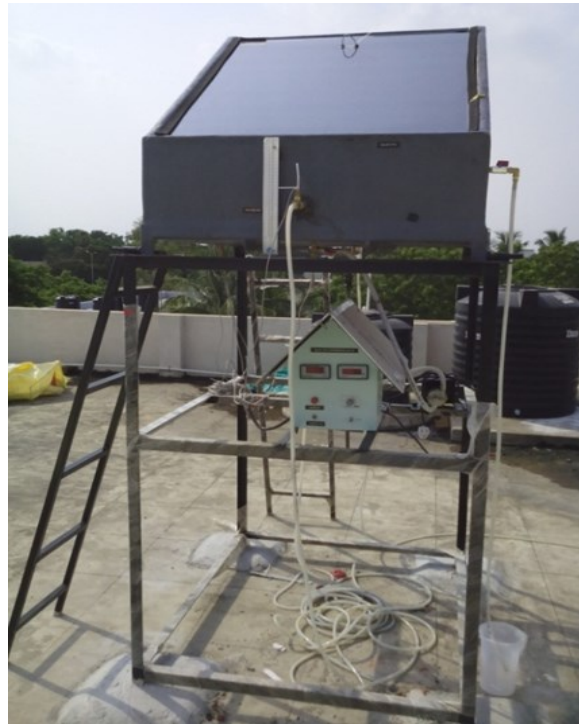
Figure 1b: Photograph of the working solar still.
